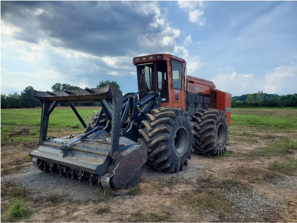
Figure 1: A forestry mulcher mounted on a Barko tractor found on site.
