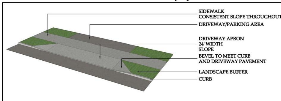
All new driveway aprons should provide a walking surface, where sidewalks are available, with a minimum two percent cross slope for a minimum width of four feet.
