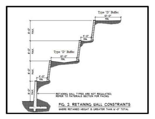
Type "D" buffer (see Article 11). Retaining walls which are separated by a building, a road, or a parking area of at least ten (10') shall be exempt from the planting requirements. See Fig. 2 below.
